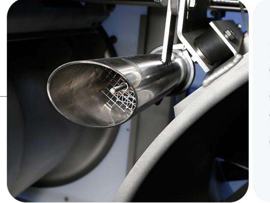
Foam generator together with the fans distribute detergent inside the freezer for an efficient cleaning cycle.
